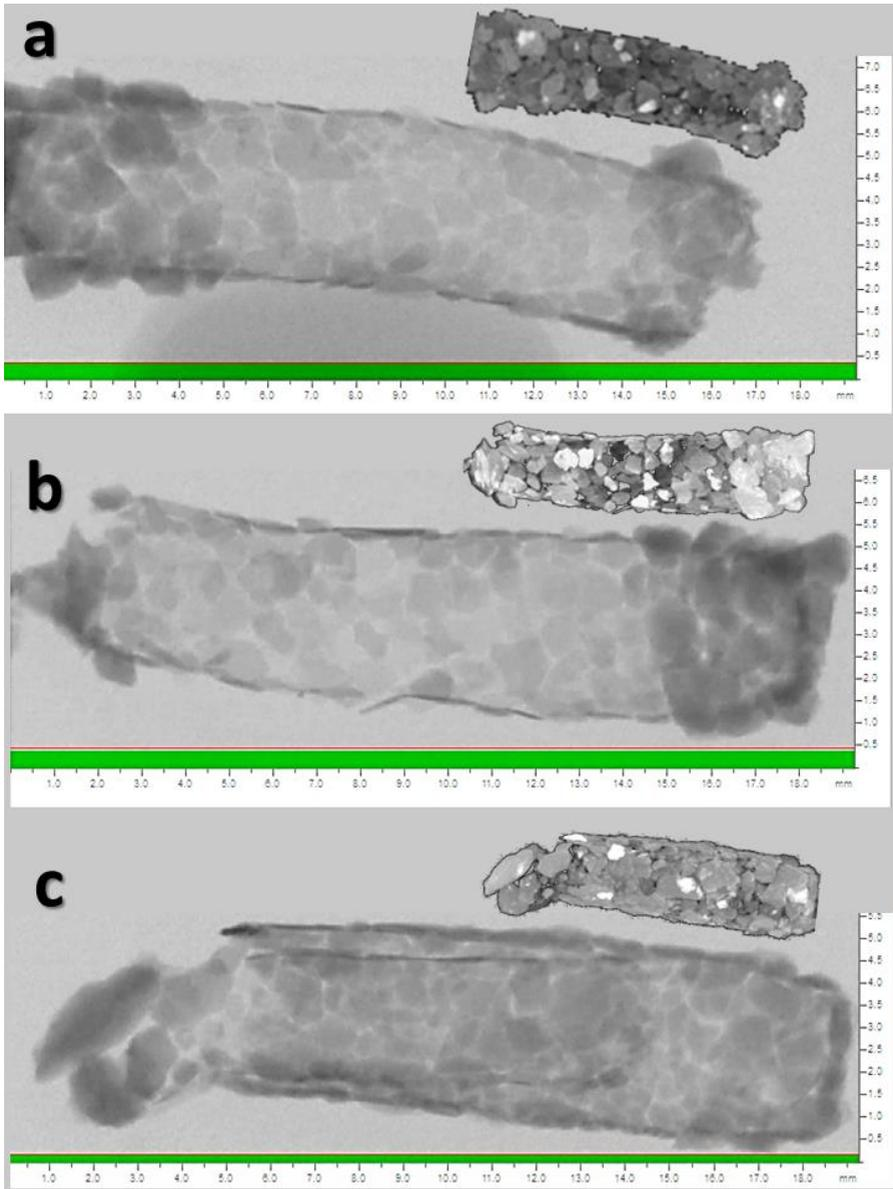
**Figure 2:** Shadow projections (x-ray) images of studied caddisfly pupal cases (a: case #4, b: case #5 & c: case #6). On the top of each x-ray picture are new shadow projections images obtained with DataViewer once the images were reoriented and reopened (see text for details). (a, b, c: Source Voltage = 64kV, Source Current = 100  $\mu$ A, Pixel Size = 15.06  $\mu$ m).
