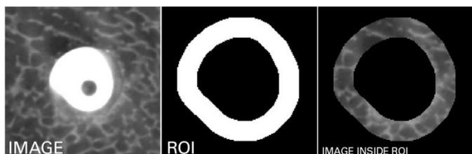
*Small part of a cross section through the implant, the annular ROI and the bone formation inside the ROI.*
