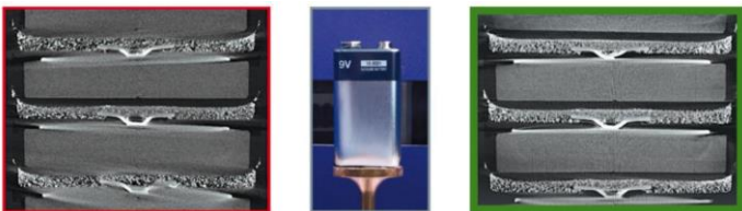
Two vertical slices through a 9 V battery are shown from scans made with the SkyScan 1275. For the image on the left, a circular trajectory was used, for the one on the right a helical scanning trajectory. An exact reconstruction algorithm was used for the reconstruction of the helical scan data.
