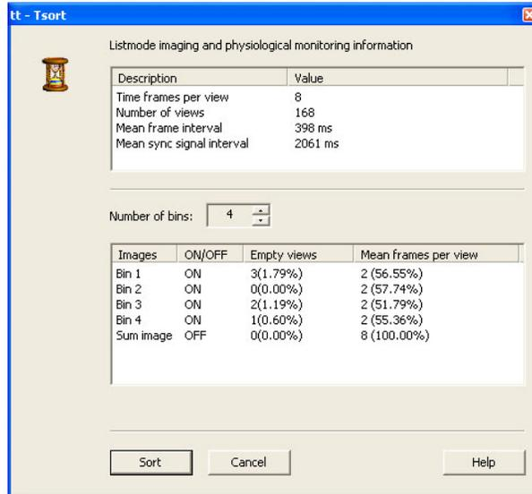
Tsort can be invoked by drag-and-drop, double-click or by other SkyScan programs. Multiple instances are allowed: care should be taken when one works on the same dataset with multiple instances of Tsort. The original projection image dataset will not be modified in any way by Tsort. The sorted datasets, or the bins, are stored in the same directory as the input listmode data. They are ready for reconstruction and further processing. These sorted datasets have a fixed name convention as well:
