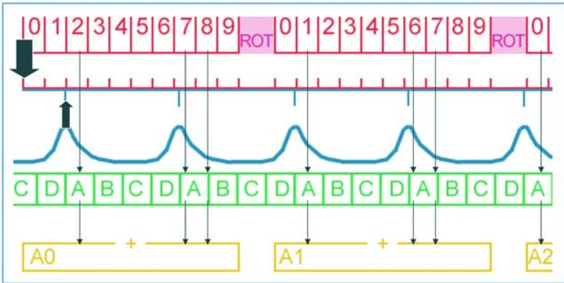
Tsort performs the same procedure for all four time bins and finally creates four new sets of angular projections: A0,A1,A2,...; B0,B1,B2,...; C0,C1,C2,...; D0,D1,D2,... as shown in the following picture:
