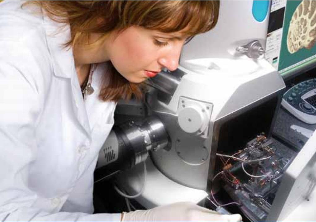
Micro-CT for SEM adds true 3D microscopy to your SEM – regardless of manufacturer and model. Micro-CT for SEM extends the surface information gained with conventional SEM imaging by allowing a unique insight into the specimen's internal microstructures – nondestructively and with ease of use.
